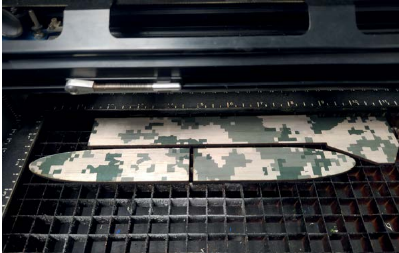
Above Cut sections of the larger EXO-B model in the laser cutter
