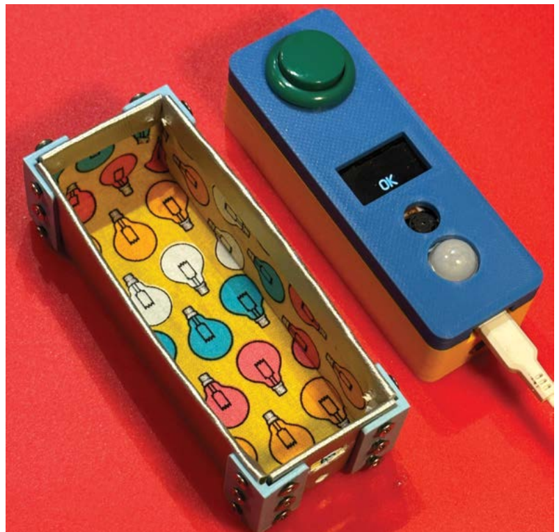
Figure 3 ♦ The holes in the plates have a larger 'countersink' hole at one side. Make sure you screw the bolt into this larger hole so that the head is slightly recessed
