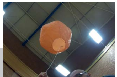
Figure 13 → CDAS-2 at launch with its tiny FPV camera, video transmitter, and battery payload
