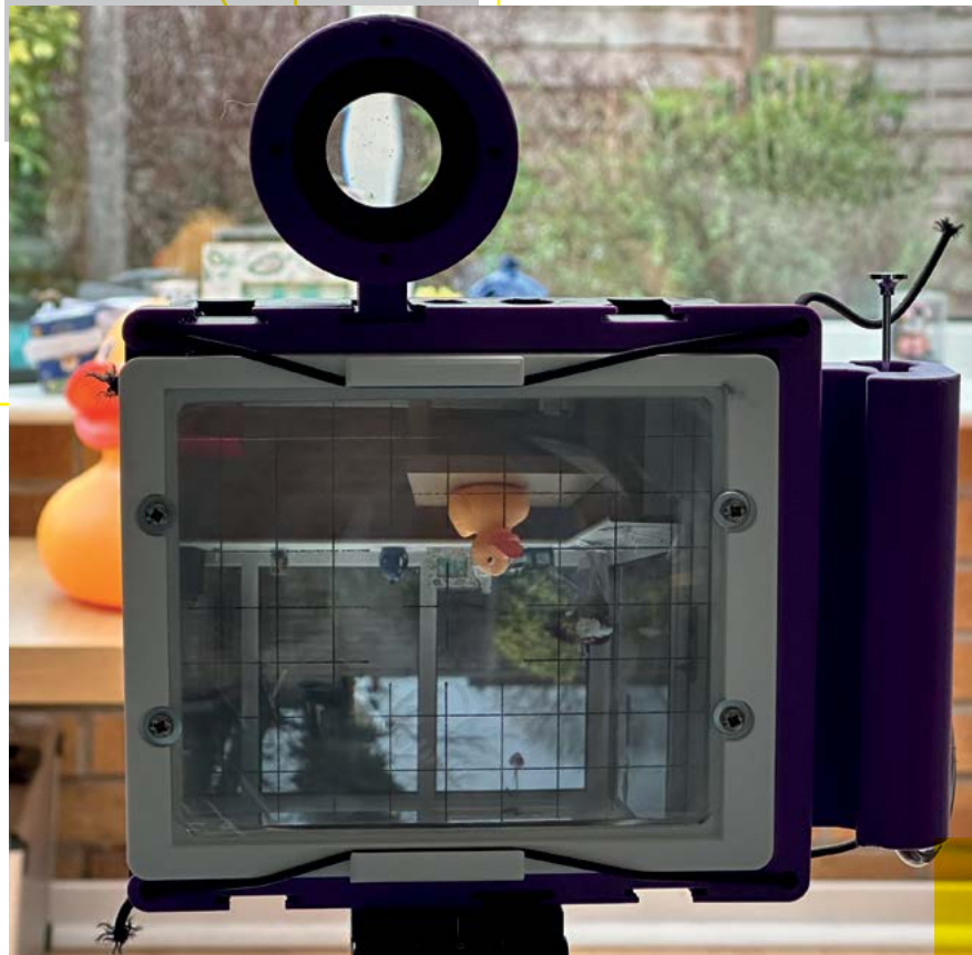
Figure 2 You can add a Fresnel lens on top of the ground glass to make the image brighter
