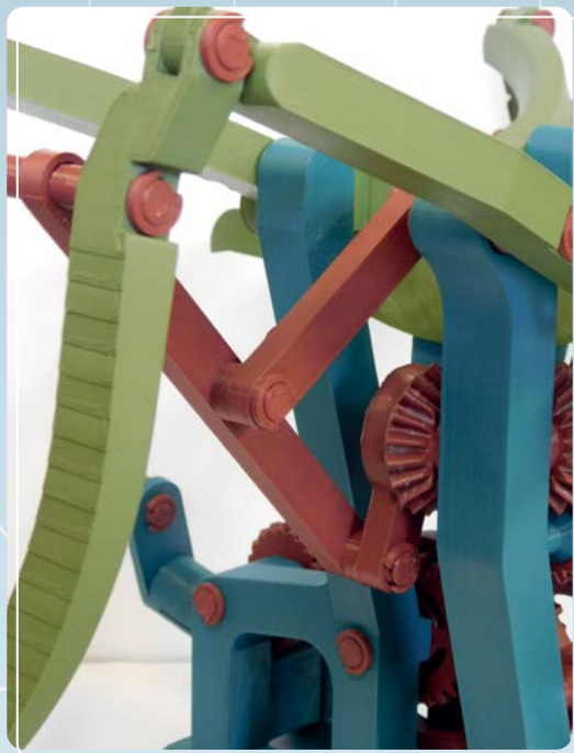
Above ♦ The linkage is a bit stiff in practice, so you'll need some sandpaper and patience to get it flapping
