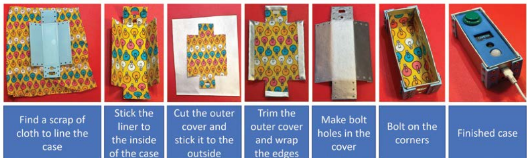
Figure 5 ♦ You can use a 1/8-inch drill bit to cut holes in the outer for the corner fixing bolts. Alternatively, you can cut the outer cover material to shape first and punch holes in it before sticking it onto the stiffener
