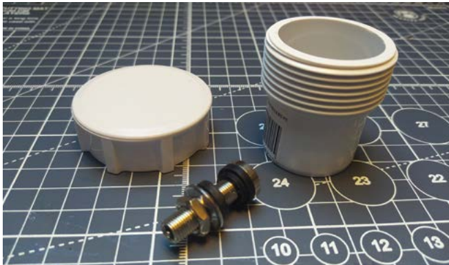
Figure 2 ⬆ A threaded Schrader-style valve with rubber seals
