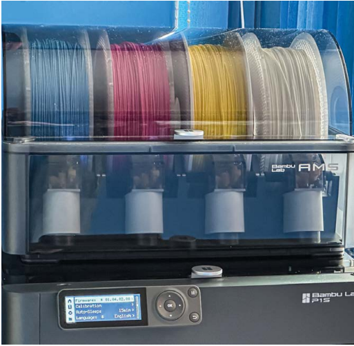
Figure 2 ♦ The selector has been loaded with cyan, magenta, yellow, and white filaments to make a colour lithophane
